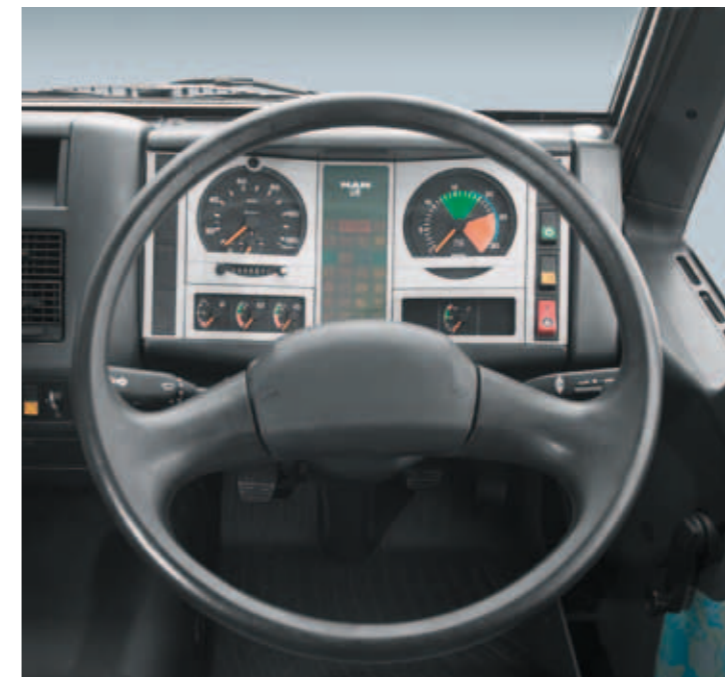
Steering wheel adjustable in height and angle.
